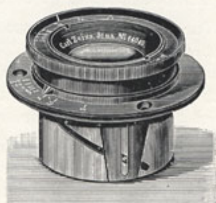
Special Mount A with Focussing Adjustment and Iris-diaphragm for Stand Cameras with fixed Extension, the objective projecting inwards through the camera front.
