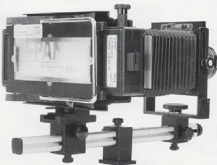
REARVIEW OF V-PAN, FILM MAGAZINE INSERTED. NOTE DOVE-TAIL SLIDE, AND HOLE IN BEATTIE INTENSCREEN FOR READING FILM NUMBERS.
