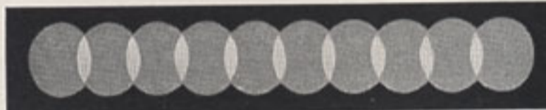
The Graflex focal plane shutter transmits all the available light during the entire exposure.
