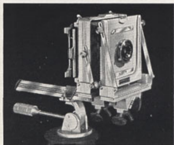
To prevent the picture from being cut-off when wide-angle lenses are used, the camera front and back may be shifted forward on the bed.
