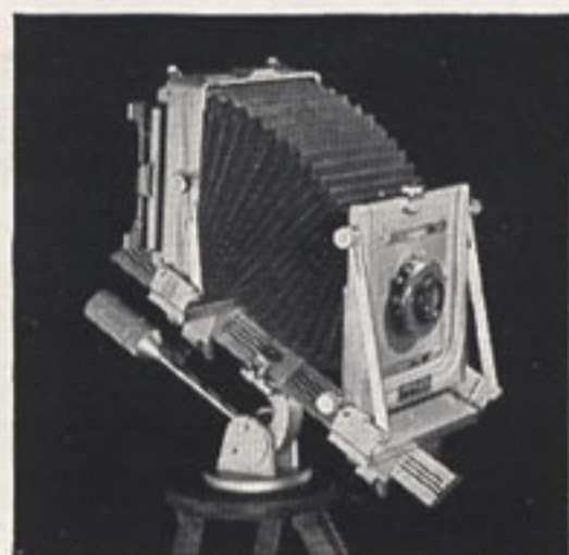
When shooting downward, linear perspective may be altered by tilting both lens and film backward to create parallelism of vertical lines.
