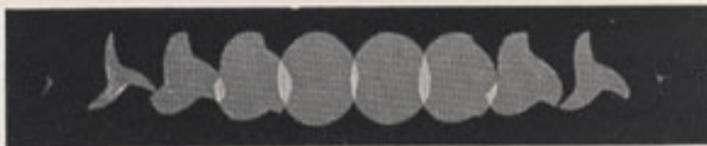
The between-the-lens shutter is wide open during only the fifth and sixth flashes.
