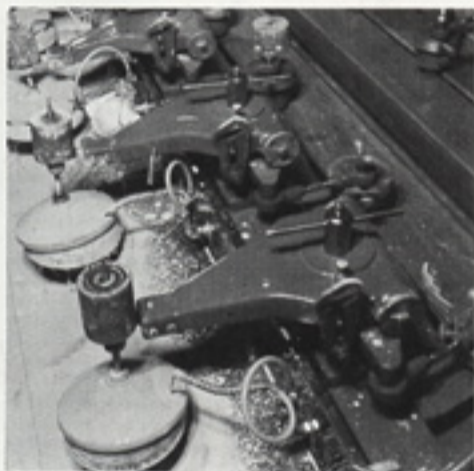
Automatic lens polishers. Hundreds of these units, large and small, are employed at Fuji's Omiya Factory.
