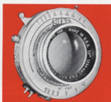
L-113 254mm (10") Caltar lens f/6.3 — f/45 Ilex synchro M/X Shutter, T.B., 1 second to 1/150th press focus. (This focal length is superb for portraiture.)
