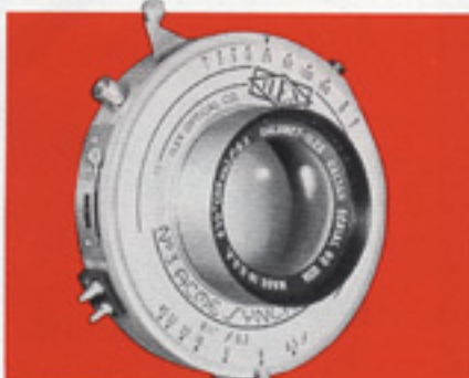
L-111 215mm (8½") Caltar lens f/6.3 — f/45 Ilex synchro M/X shutter T.B. 1 second to 1/150th press focus.
