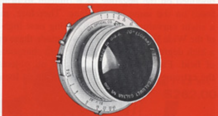
L-120 20" Caltar lens in #5 Universal M/X Shutter f/7.0 — f/45, T.B. 1 second to 1/50th, press focus.
