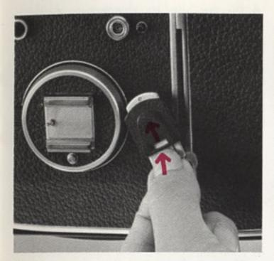
**b** To remove the neck strap, grasp the strap, as shown in the photograph, and with the finger-tip, press down the spring pressure plate, and push the strap metal into the plastic holder, unlocking the strap from the strap stud.
