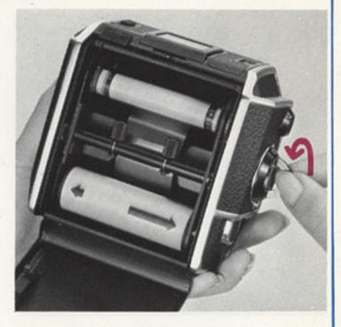
The procedure, here, is the same as that for loading film with the film back coupled to the camera up to loading film onto the film holder insert.
