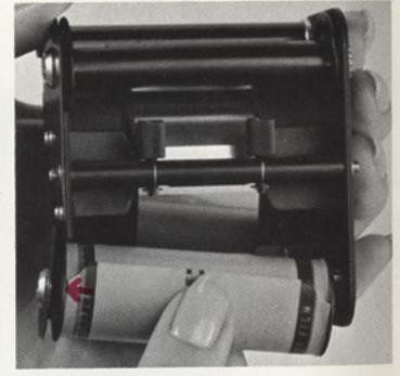
c Spool holders are located at the top and bottom of the insert. The top holder is for the empty take-up spool and the bottom holder is for the fresh film spool. A spring pressure plate is located on one side of the spool holder. Insert one end of the empty take-up spool against this plate and, while pressing the plate out, insert the other end of the spool into place.
