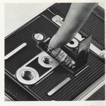
c A red "+" mark and a blue "-" are stamped inside the battery chamber. Insert the battery matching these marks with the "+" and "-" marks on the battery, placing the negative side of the battery into the chamber first, pushing the positive side into place, and then closing battery chamber cover. The shutter will not operate if these polarity marks are mismatched.
