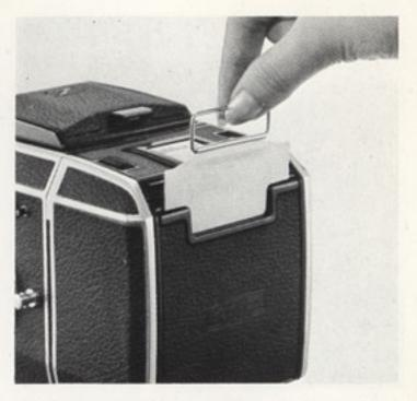
\* After attaching the film back to the camera body, always withdraw the dark slide and insert it into the dark slide pocket. Shutter release is not possible with the slide inserted, and there is the possibility of the film back falling from the camera if it is carried in this state.
