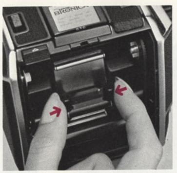
**b** Opening the back cover of the film back reveals the film holder insert, which has two center-positioned knobs. Press these inward, releasing the lock, and remove the insert from the film back body.
