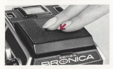
**b** To attach the focusing hood, insert the focusing hood into its frame atop the camera, as shown in the photograph, and press down and lock it at the front.
