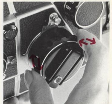
\* The crank stops after it is turned twice, but if additional pressure is applied downward it will continue to turn. This is not a malfunction but the operation of a special safety feature. Applying additional pressure after the crank stops following two full turns is not recommended.
