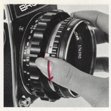
c To remove a lens, turn the focusing ring fully clockwise, press and hold the lens release lever with the thumb on the left-hand side of the lens, turn the lens to the left (counterclock-wise) until it stops, and withdraw the lens,
