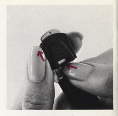
a To attach the strap to the camera, press and hold down the spring plate on the strap metal, as shown in the photograph, and slide the plastic holder toward the strap using the metal protrusion atop the plastic holder. The hole on the reverse side of the plastic holder opens. Insert the neck strap stud on the camera body into this hole, and pull the strap toward you, locking the strap onto the neck strap stud.
