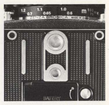
Two threaded holes are provided beneath the camera for attaching a tripod. The large, 3/8-inch-diameter hole is for European-make tripods, and the small 1/4-inchdiameter hole is for Japanese and American-make tripods.
