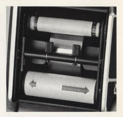
f Wind the film shutter knob/crank and advance the film leader paper to the film start point (the arrow mark on the film), and align the film start point and the red dot on the film holder insert,
